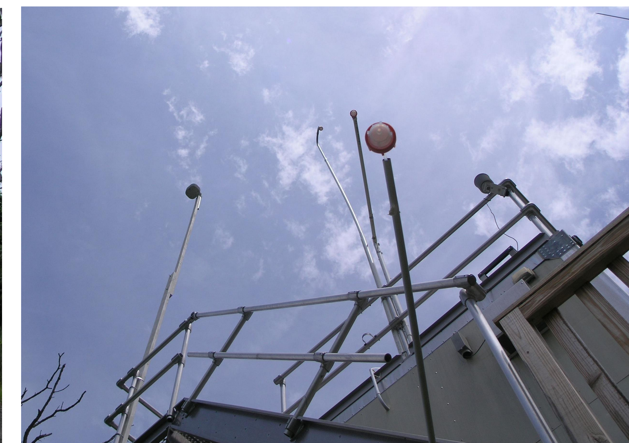
Figure 4. Three O 3 test array inlets from ground level.
